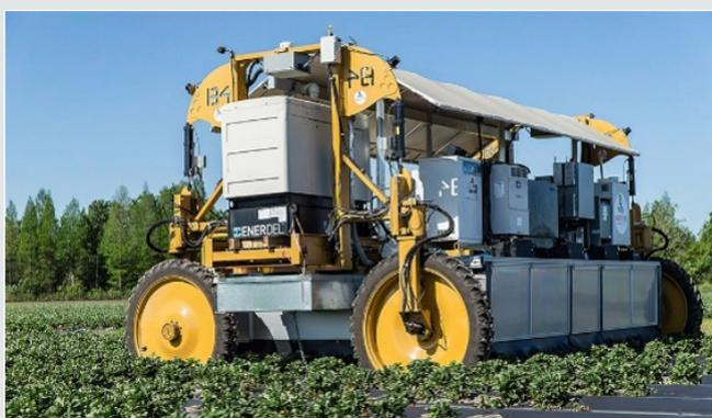
**Figure 1:** Illustrates Harvesting CROO's machine is headed for farms in Florida and California. Image Credit: Image courtesy of Harvest CROO Robotics [1].
