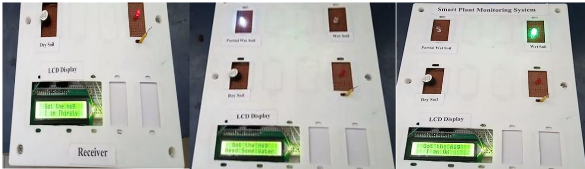
Fig (i): User indicator for dry soil Fig (j): User indicator partial wet soil Fig (k): User indicator for wet soil
