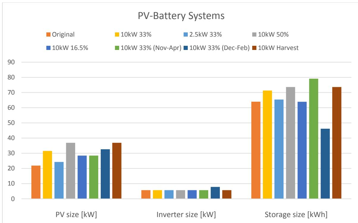
**Figure 21. Optimal generation sizing for PV-battery systems**
