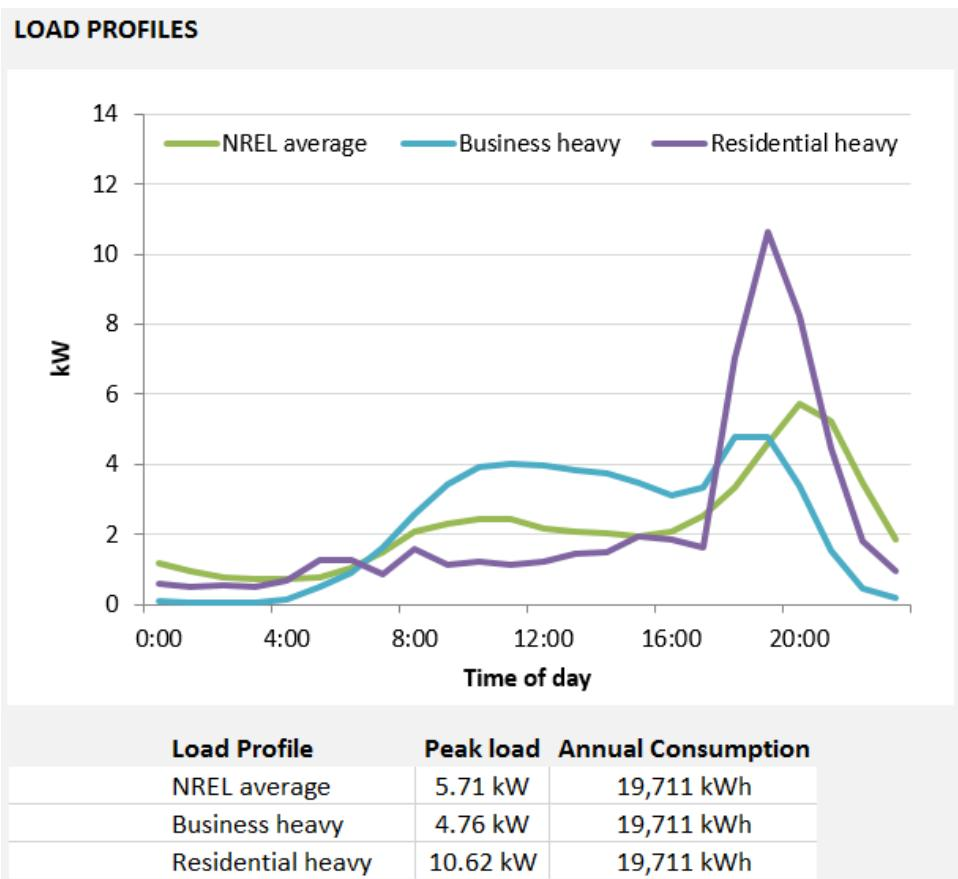
**Figure A2-2. Load profiles used in LCOE analysis**
