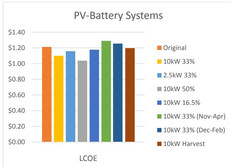
**Figure 19. LCOE of PV-battery systems (\$/kWh)**
