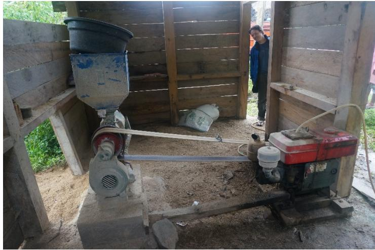
**Figure 10: Diesel powered milling machine**
