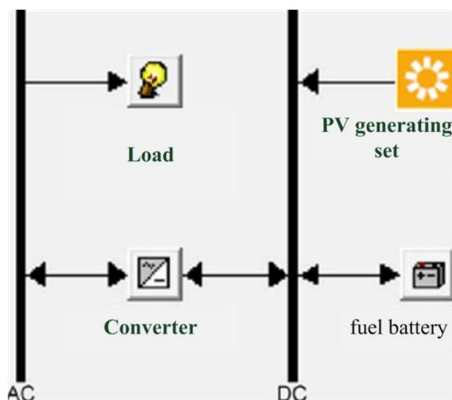
Figure 6. PV-based independent micro-grid system.
