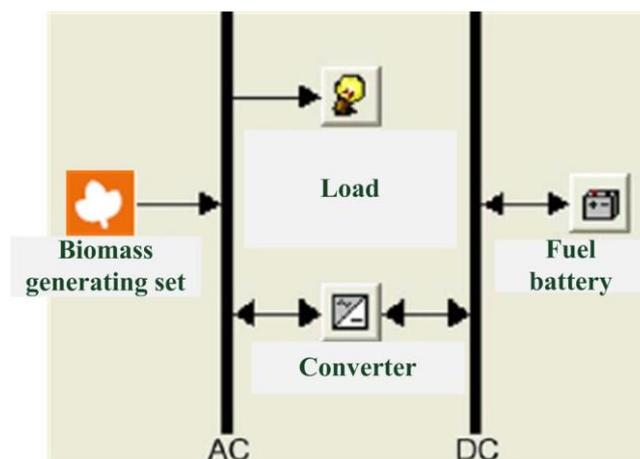
Figure 7. Biomass-based independent micro-grid system.
