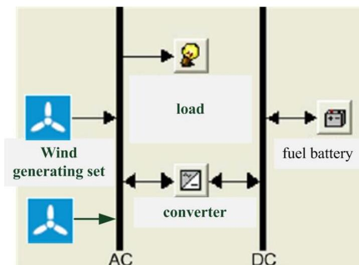
Figure 5. Wind -based independent micro-grid system.
