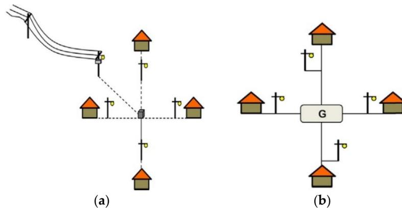
**Figure 1.** Schematic diagram of two modes for rural electrification. (a) Grid extension; (b) Micro-grid.
