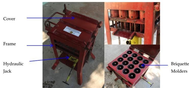
**Figure 1.** The hydraulic jack-driven briquetting machine utilized in the briquette production test.
